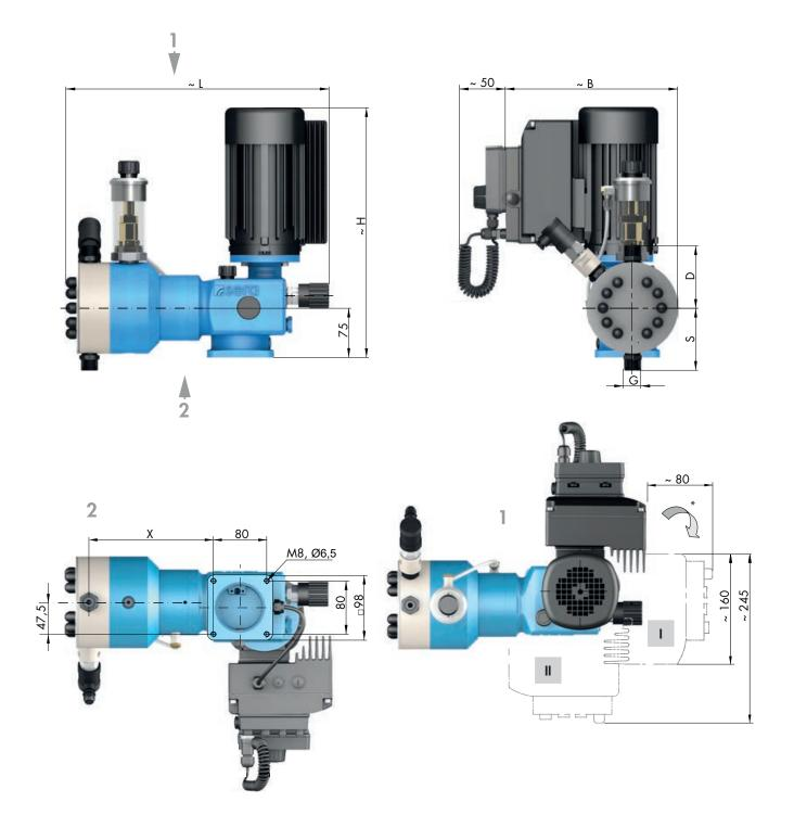
\* Drive with electronics can be rotated throughout 90° each and can be put to the positions I and II. (release the motor fastening screws, put the motor carefully to the desired position and fasten with screws again).
