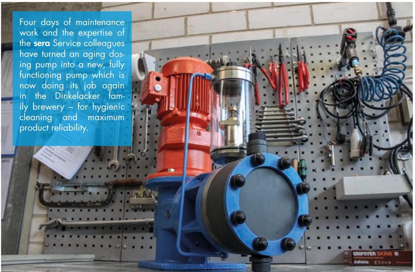
Four days of maintenance work and the expertise of the **sera** Service colleagues have turned an aging dosing pump into a new, fully functioning pump which is now doing its job again in the Dinkelacker family brewery – for hygienic cleaning and maximum product reliability.
