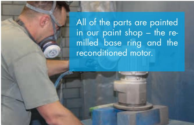
All of the parts are painted in our paint shop – the re-milled base ring and the reconditioned motor.
