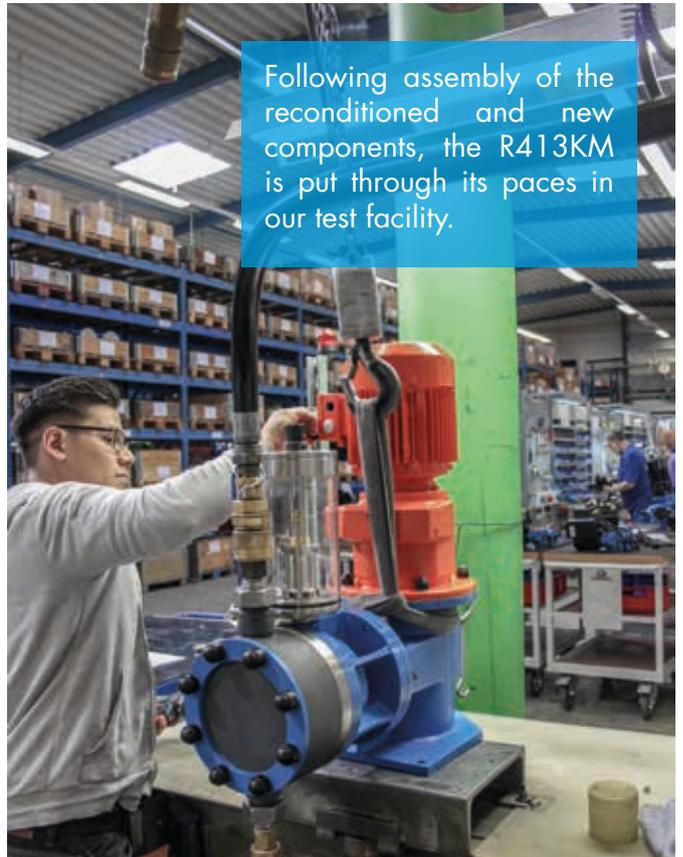
Following assembly of the reconditioned and new components, the R413KM is put through its paces in our test facility.
