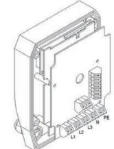
■ Insert the mains pipe through the cable fitting M20 from below into the housing.
