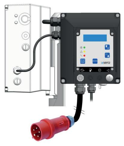
The mains connection requires 3~ 400V + neutral conductor + protective conductor. The leakage current against earth amounts to approx. 7 mA. Recommended protection: 3-poles automatic fuse C10A.
