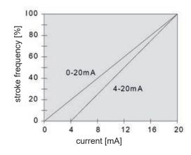
The anlog control signal can be adjusted according to needs. This is, for example, necessary if a connected regulator provides a limited output signal.
